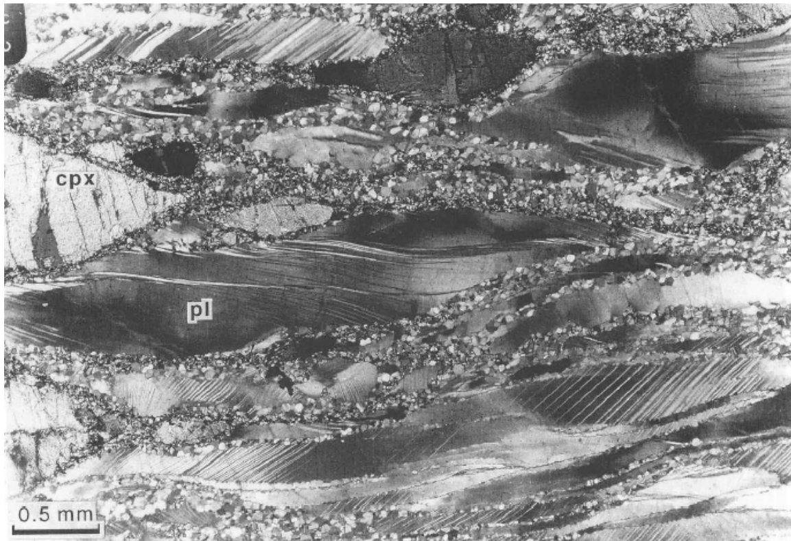
Jotun nappe amphibolite-facies anorthosite mylonite with plagioclase ribbon porphyroclasts showing undulatory extinction, twinning and clinopyroxene recrystallized into amphibole (Ji, 1998)
