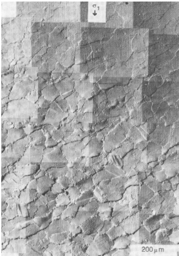
displaced grains in split cylinder indicate GBS in Carrara marble (Rutter, 1995)
