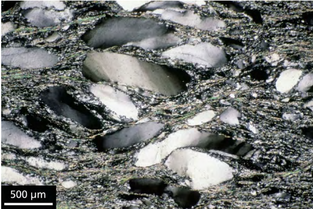
Regime 2. Heavitree quartzite deformed at greenschist conditions by simultaneous subgrain rotation recrystallization and solution–precipitation. Detrital quartz grains are flattened, stretched, and bent in a fine-grained quartz-mica matrix. A NE-SW shear band deforms the dominant foliation and indicates top-to-the-left sense of shear. (Tullis et al., 2000)
