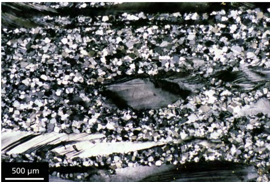
Jotun anorthosite moderately deformed at 700°C; regime 2 (Tullis et al., 2000)
