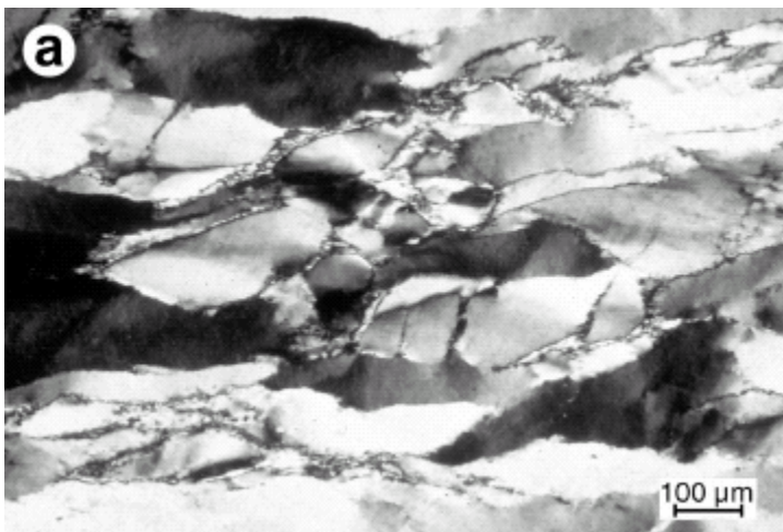
Regime 1 BLG at 310°C porphyroclasts show undulatory extinction and serrated grain boundaries (Stipp et al., 2002)
