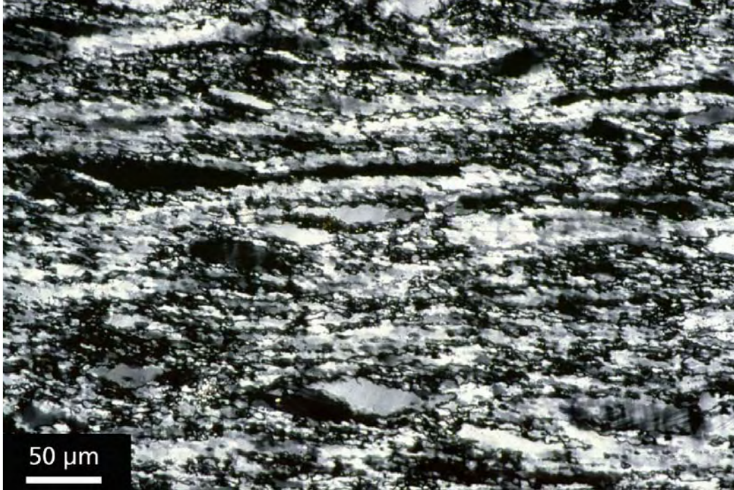
Regime 2, 50% shortening and simple shear at 800°C and 10^{-5} \text{ s}^{-1} (Tullis et al, 2000)
