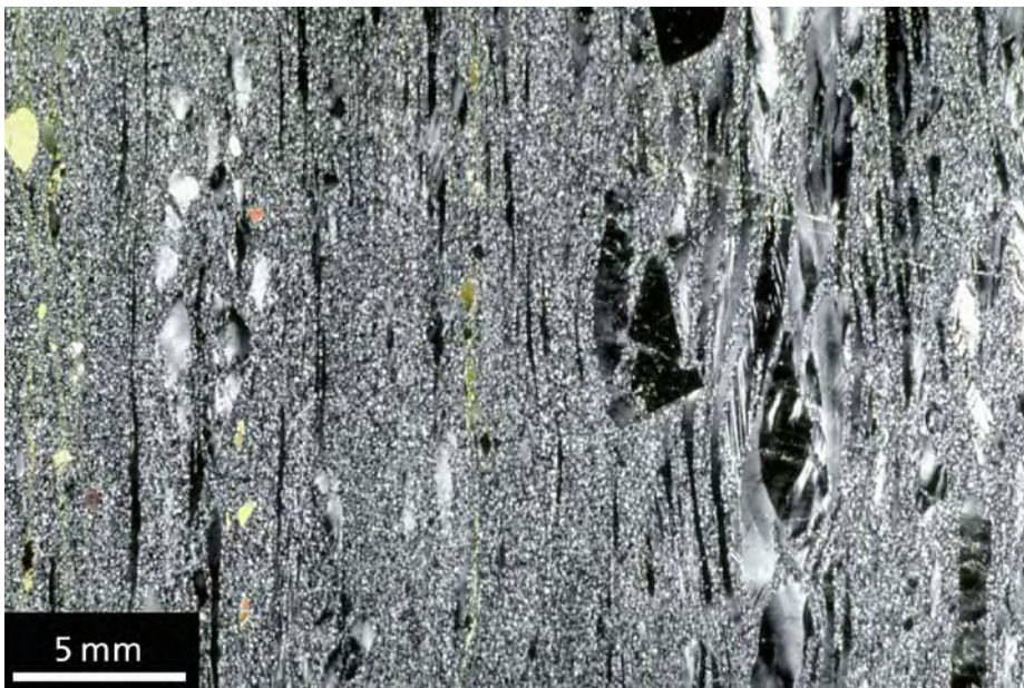
Jotun anorthosite strongly deformed at 700°C; regime 2 (Tullis et al., 2000)
