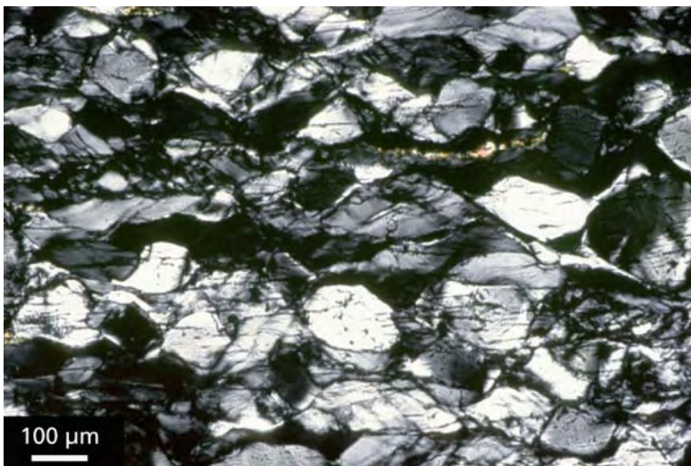
Enfield aplite shortened 35% at 725°C and 10^{-6} \text{ s}^{-1} (Tullis et al., 2000). At these conditions quartzite deforms by BLG (regime 1) dislocation creep and is weaker than anorthosite, which deforms by cataclastic flow. This aplite shows that the isolated quartz was stronger than the feldspar, because in regime 1 dislocation creep, the recovery process is bulging recrystallization, which can only occur if there are quartz–quartz grain boundaries.
