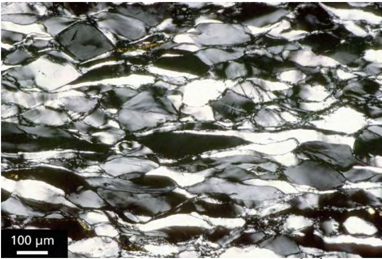
Enfield aplite shortened 60% at 900°C and 10^{-6} \text{ s}^{-1} . Quartz deforms by SGR (regime 2) dislocation creep and the feldspars deform by BLG (regime 1) dislocation creep. Because dislocation climb is easy in quartz, it undergoes homogeneous flattening; some grains show sub-basal deformation lamellae, and recrystallized grains formed by SGR are observed especially along some grain boundaries. The feldspars are stronger and deform less homogeneously, including necking (Tullis et al., 2000)
