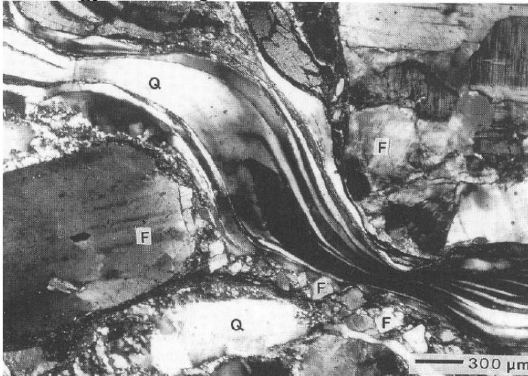
Borrego Springs mylonite shows ductile (Regime 2) quartz and brittle feldspar (Simpson, 1998)
