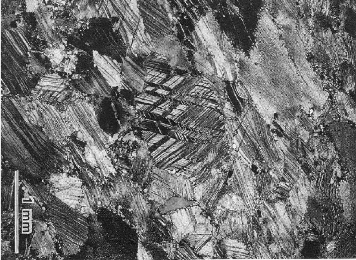
coarse-grained Palm Canyon marble showing twinning, kinking, and grain-boundary recrystallization (Erskine & Wenk, 1998)
