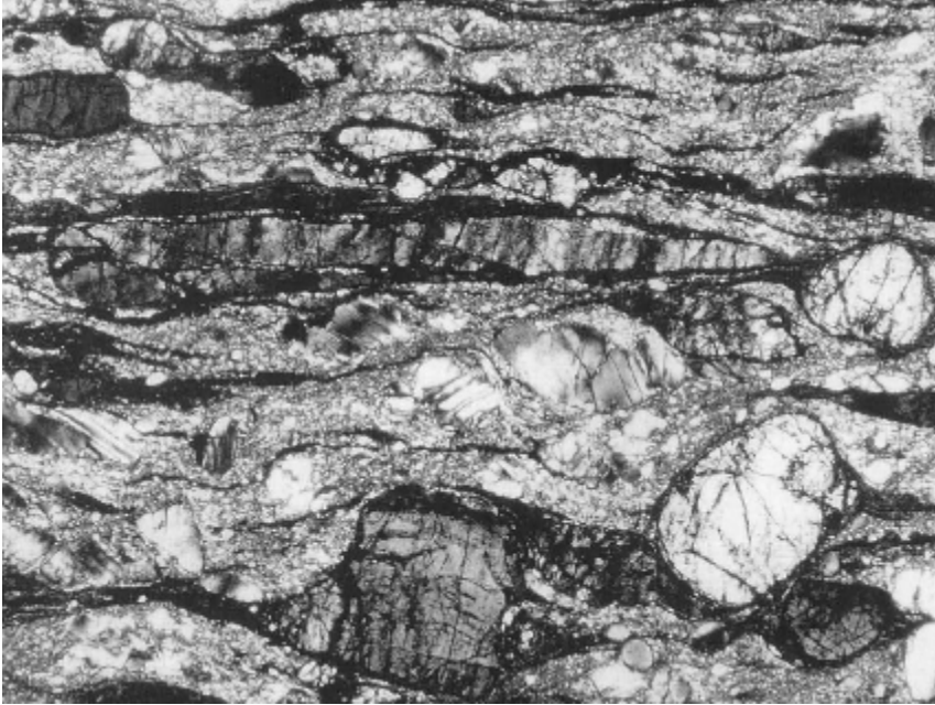
plagioclase recrystallized to very fine grain size; orthopyroxene locally elongated by slip (Brodie, 1998)
