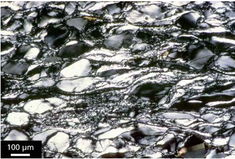
Enfield aplite shortened 85% at 900°C, 10^{-6} \text{ s}^{-1} ; recrystallized ribbons of quartz, feldspar augen with tails (Tullis et al., 2000).
