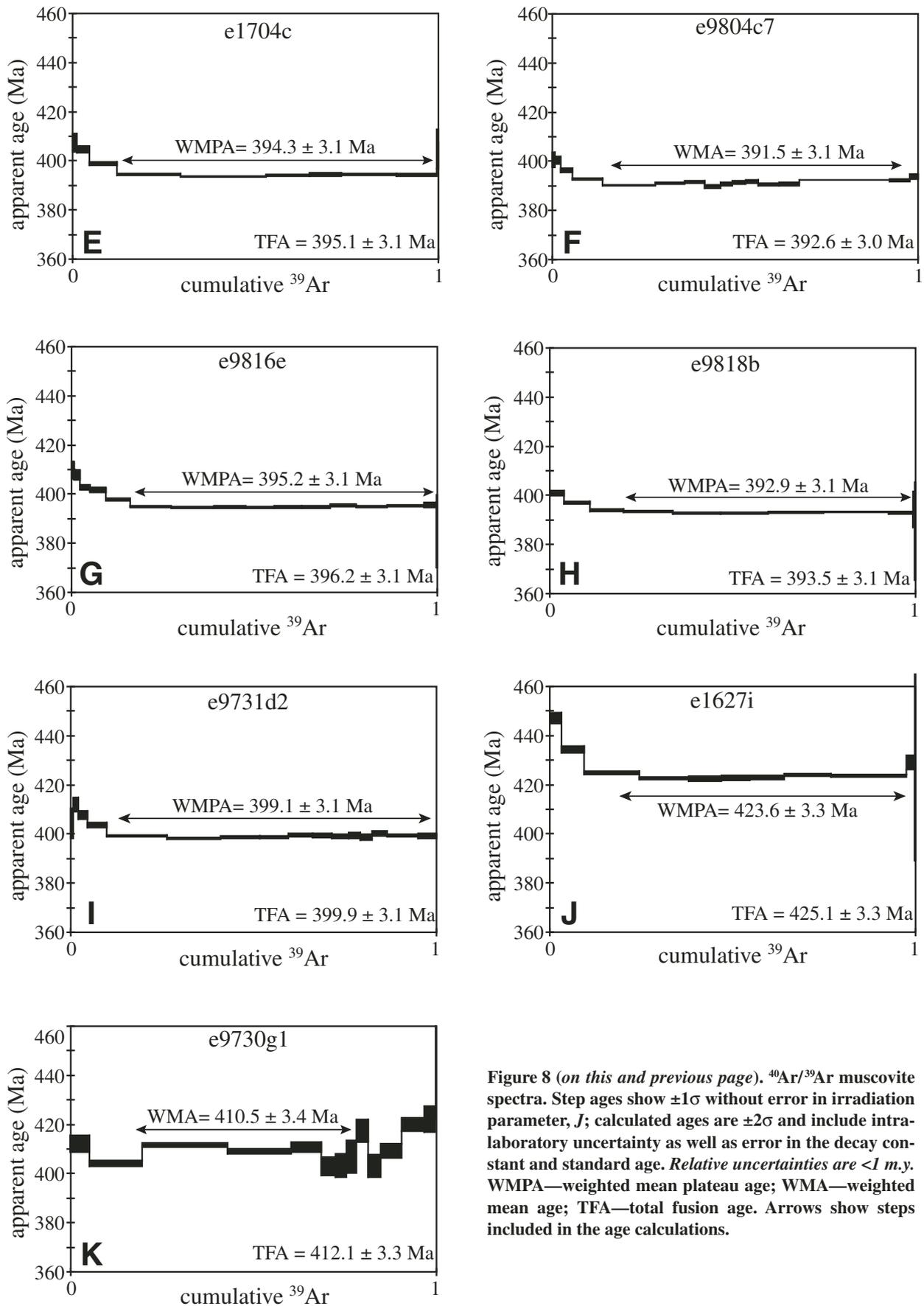
Figure 8 (on this and previous page).  $^{40}\text{Ar}/^{39}\text{Ar}$  muscovite spectra. Step ages show  $\pm 1\sigma$  without error in irradiation parameter,  $J$ ; calculated ages are  $\pm 2\sigma$  and include intra-laboratory uncertainty as well as error in the decay constant and standard age. Relative uncertainties are  $< 1$  m.y. WMPA—weighted mean plateau age; WMA—weighted mean age; TFA—total fusion age. Arrows show steps included in the age calculations.
