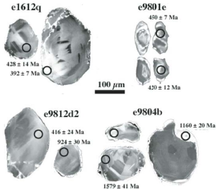
**Figure 4.** Cathodoluminescence images of representative zircons from eclogites;  $^{206}\text{Pb}/^{238}\text{U}$  spot ages are shown. Eclogites in the western part of the study area (samples e9812d2, e1612q) exhibit recrystallized textures, whereas eclogites from farther east show oscillatory or sector zoning (samples e9804b, e9801e).
